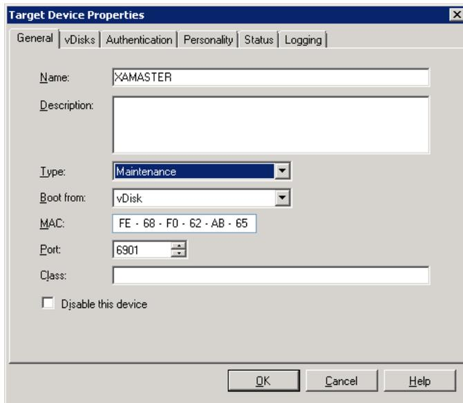
Within the Provisioning Services console open the properties of the “Master” server and change the **Type to Maintenance**. Click **OK**.
