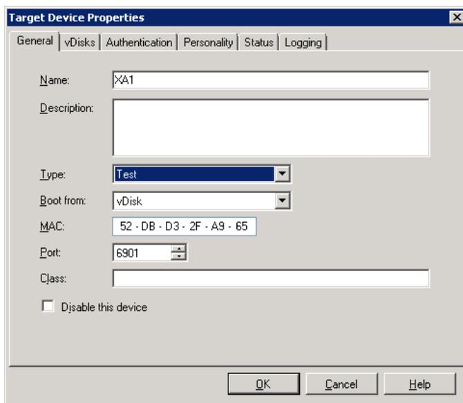
Open the properties of the Target Device you want to test the new vDisk version on and change the Type to **Test**. Click **OK**.
