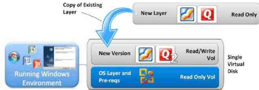
Logical example of layer versioning
