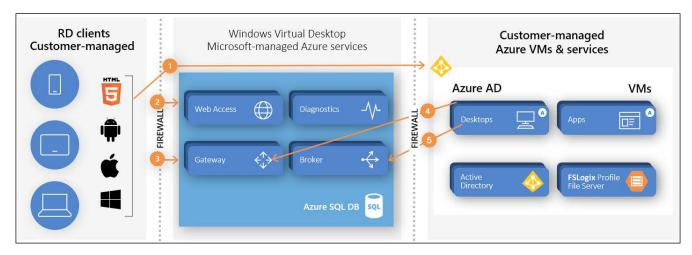
Figure 3: The connection flow process of Windows Virtual Desktop
