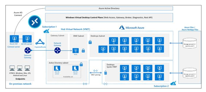
Figure 2: A typical architectural setup for Windows Virtual Desktop
